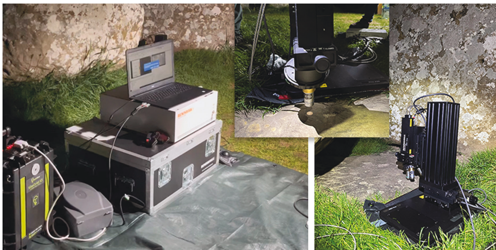
Figure 2: A versatile portable Raman laboratory. The Virsa Raman analyzer at Stonehenge, powered by a portable battery pack (left). The flexible Virsa SB200 stage carefully positioned close to the Altar Stone (right). The inset shows the Virsa probe focusing on a region of the Altar Stone.
