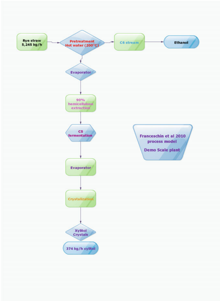
Fig. 9.5 Xylitol production through demonstration plant (Franceschin et al. 2011)
