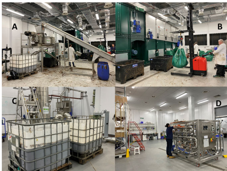
Fig. 9.2 Pilot-scale processing of pretreated biomass at Aberystwyth University biorefining centre. a Liquid/solid separation by screw press; b counter current washing solids to maximise C5 recovery; c recovered hydrolysate; d C5 sugar concentration by membrane filtration
