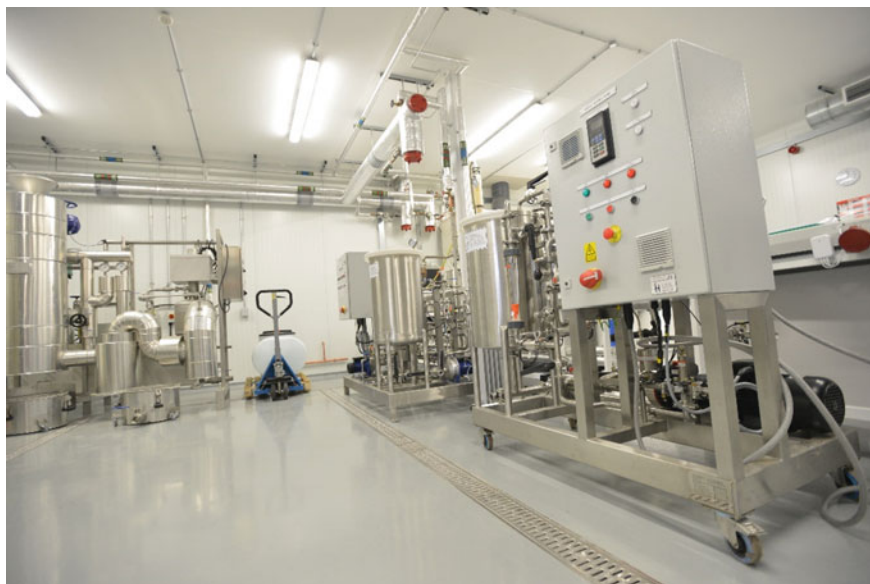
Fig. 9.1 BEACON Pilot plant with pilot-scale steam explosion rig and pilot-scale membrane purification systems ( http://www.beaconwales.org )
