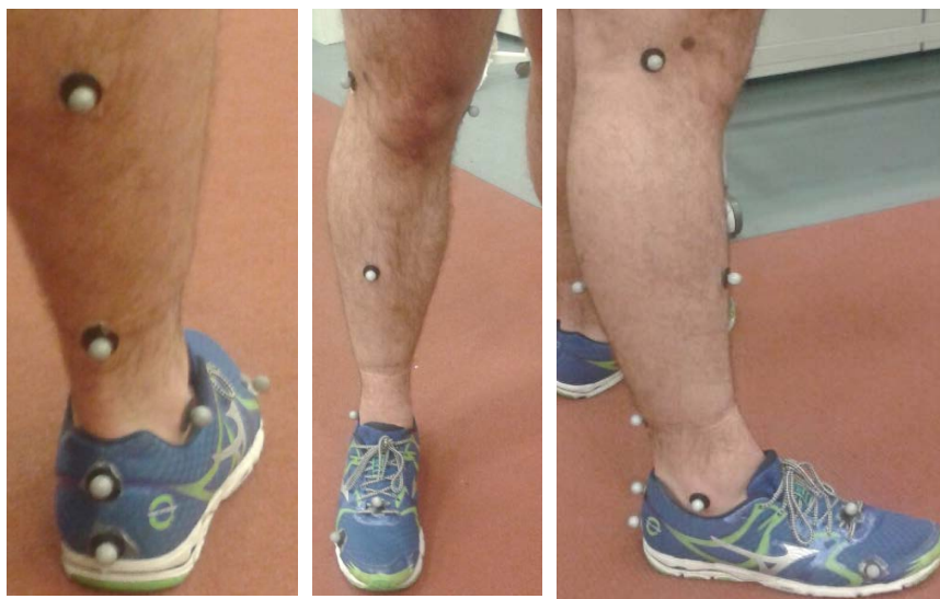
Figure 1: Images identifying marker placements used in the moment and moment arm calculation.
