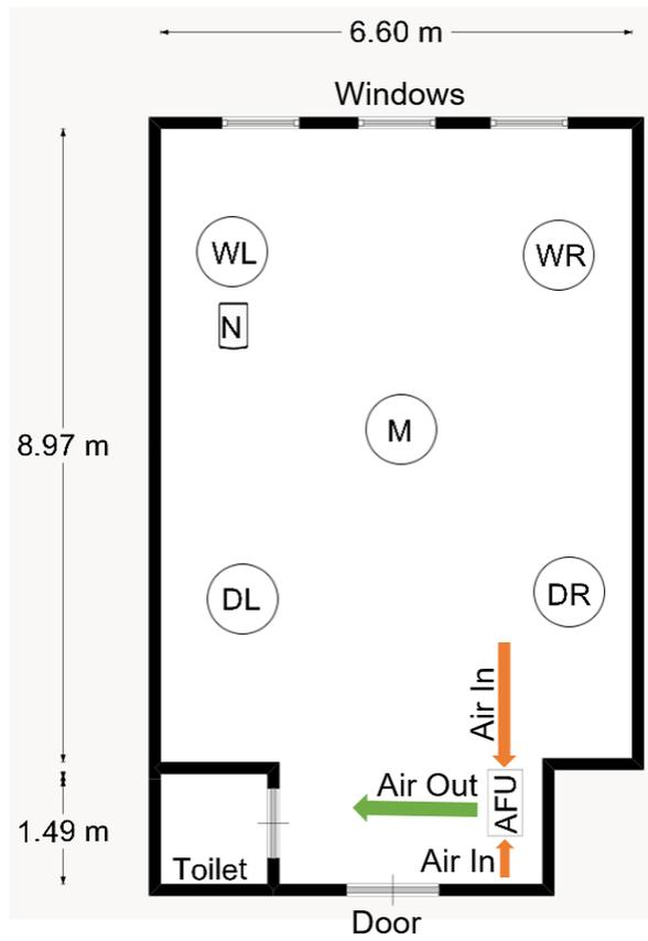
**Figure S1.** Schematic of ward showing the locations of the particle sensors. WL, window-side left; DL, door-side left; WR, window-side right; DR, door-side right, M, middle; AFU, air filtration unit; N, nebulizer.
