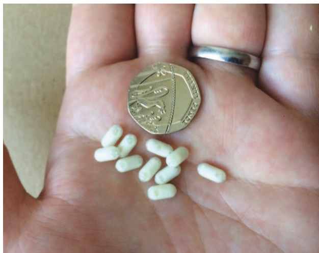
FIGURE 2. Mini-capsule MRI device markers pictured near a 20 pence coin (21 mm in diameter) for size comparison.
