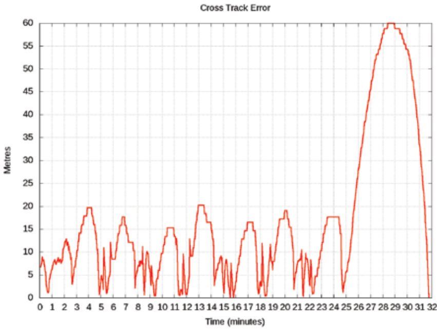
Figure 11: A graph showing the cross track error in metres against time using only the heading controller. This is the same course shown in the map in Figure 9.
