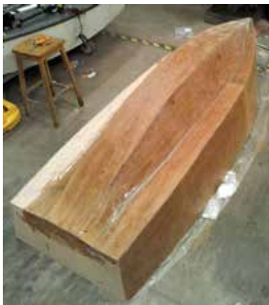
Figure 2: Minty2 in construction, showing the plywood hull material, epoxy/E-glass sheathing being applied, and the unique hull shape with transducer bump.
