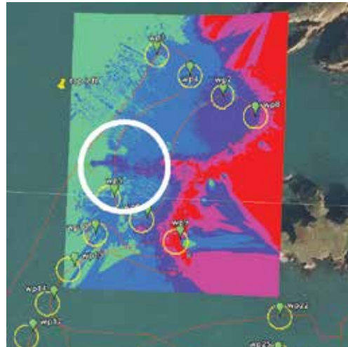
Figure 16: Interpolated bathymetry data overlaid onto an aerial photo of the Aberbach area and the wreck of the Charles Holmes . The area circled in white is believed to be the wreck site.
