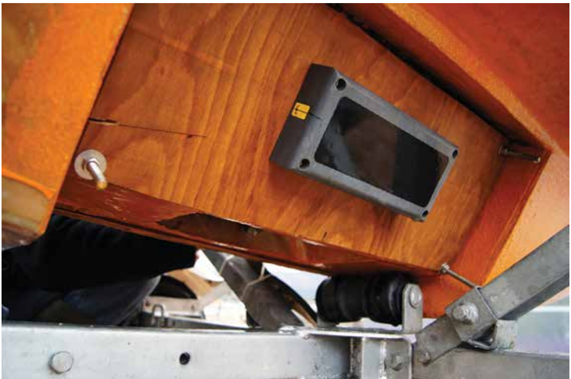
Figure 15: A photo of the smaller 468 KHz sonar transducer installed in the gap left by the 117 KHz transducer.
