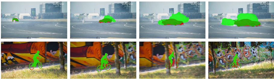
Fig. 25 Negative results due to ‘dynamic background’ (DB) and ‘shape complexity’ (SC). Top row: results predicted by RVOS (Ventura et al. 2019) on DB sequence; Bottom row: results predicted by STM (Oh et al. 2019) on SC sequence. Red masks are the ground truth masks, which are covered by the green masks (the predicted results)
