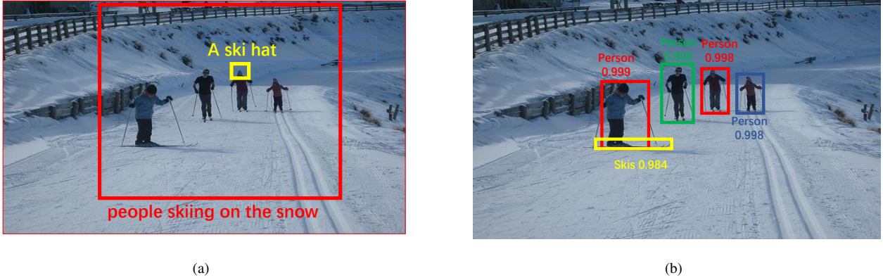
Fig. 2. An example shows the RoIs with different IoUs should be weighted differently. (a) Two RoIs and their descriptions; (b) Object detection results.
