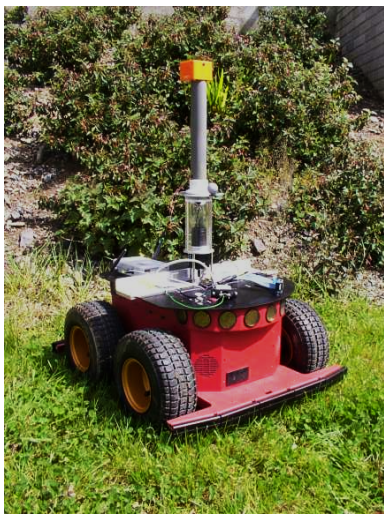
Figure 10: The outdoors robot with the camera and magnetic compass
