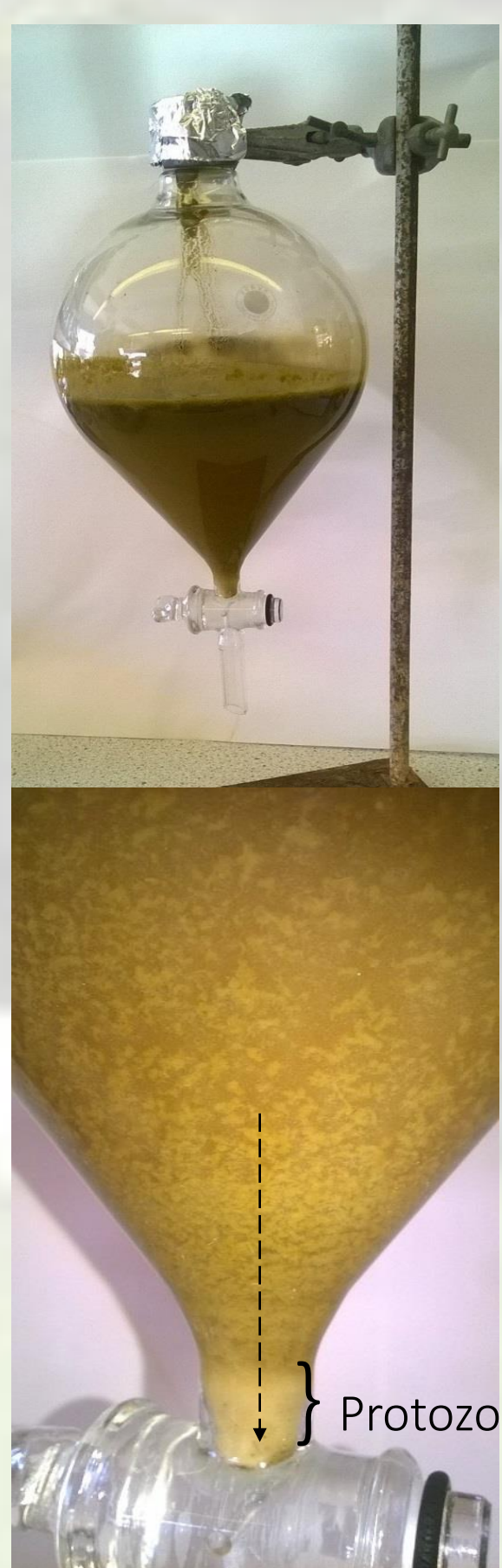
Fig.1: Separation of protozoa from rumen fluid in pear-shaped, 1L burette.
