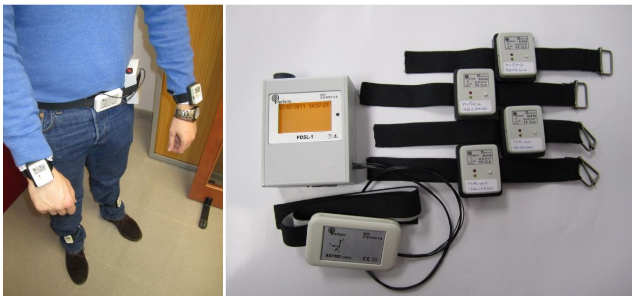
Figure 1. Sensors and data logger used for data collection and their position on the body.
