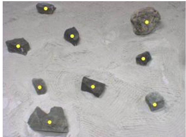
Figure 11. Input image annotated with calculated rock centroids.
