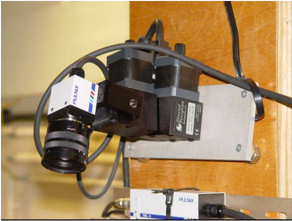
Figure 5: The Pan and Tilt "Eye" System
