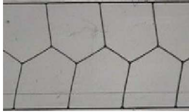
Figure 8. Snapshot of an experiment in which a 211 structure is propelled rapidly to the right along a rectangular channel (width w \approx 5\text{mm} , depth h \approx 1\text{mm} ) by an imposed pressure [3]. A dry foam in steady plug flow is observed, that is, all elements of the structure move with the same velocity V of the order of centimetres per second.
