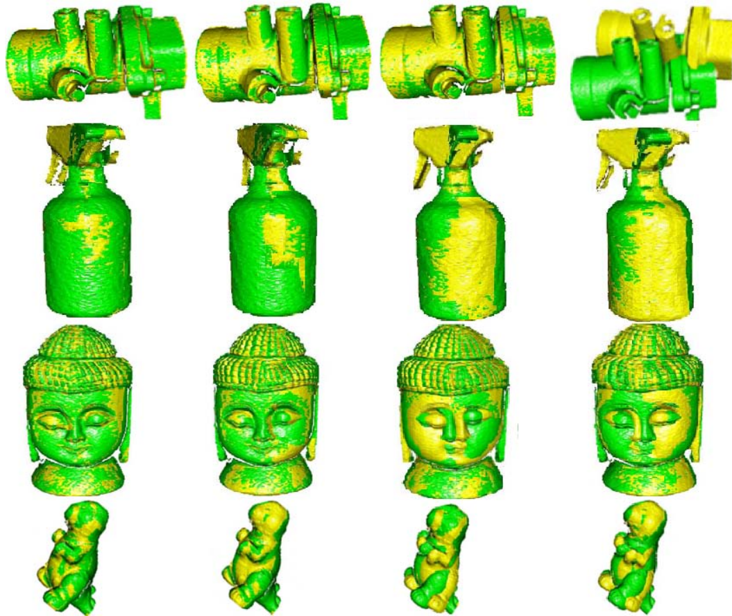
Figure 10: Registration results using the FICP algorithm of the interest points detected from different scans using different algorithms. Columns, left to right: RBS, OVBS, 3D-SIFT, and 3D-Harris. Rows, top to bottom: valve0-10, bottle144-180, buddha0-20, and dinosaur36-72.
