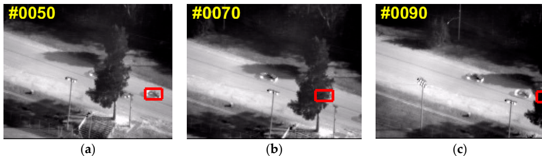
Figure 2. Tracking results of DSST: (a) tracking well without occlusion; (b) tracking failed within occlusion; and (c) model drift after occlusion.
