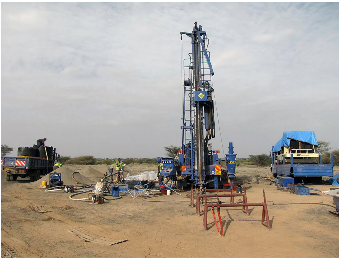
Figure 7. Photos of the HSPDP drilling operations. Left: West Turkana (WTK) site using a truck-mounted PRD Multistar drilling rig operated by Drilling and Prospecting International (DPI) used for all Kenyan drilling campaigns (photo credit: Craig Feibel). Right: Northern Awash (NAO) site using a track mounted Christensen CS14 drilling rig operated by Geosearch (now Orezone Drilling) used for Ethiopian campaigns (photo credit: Beau Marshall).
