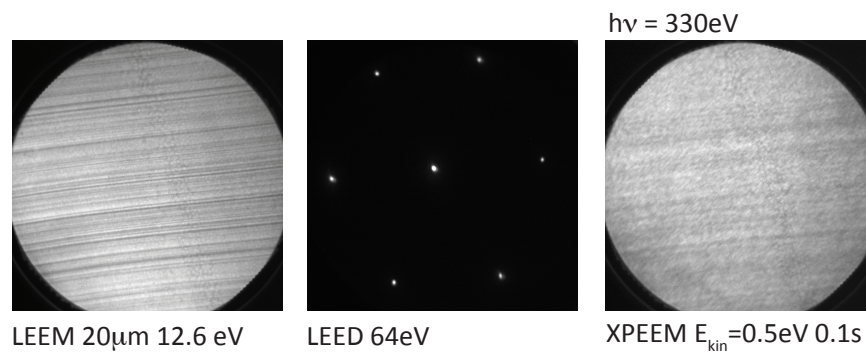
Figure 5.13 The surface following atomic hydrogen adsorption a) LEEM image of the surface shows no structural degradation of the surface following the procedure. b) LEED image shows the re-emerging (1×1) surface configuration. c) XPEEM image of secondary electrons at E_{kin}=0.5 eV image is a factor of 10 more bright than comparison to secondary images taken for previous steps.
