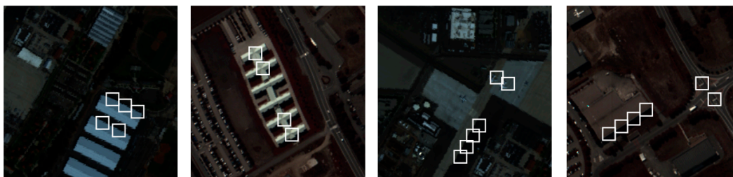
Figure 1. Similar or repeating patches (denoted by small white squares) in HSI composite images with bands 28, 19, and 10 in red green, and blue, respectively.
