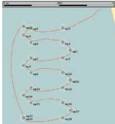
Figure 9: A map showing a survey pattern being followed using only a heading controller. The white circles around each waypoint indicate the threshold distance and the red line indicates the path taken.
