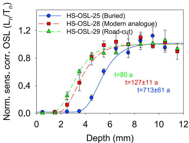
**Figure 2.** Bleaching with depth model fitted to data points of three samples with different exposure histories. Each data point is an average of at least three aliquots. Error bars represent one standard error. The curves are best fit model calculations assuming common values of  $\sigma\phi_0$  and  $\mu$  for all three samples.
