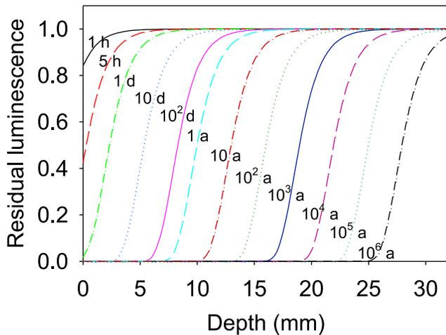
**Figure 1.** Profile of residual luminescence in a rock after a given exposure time, as predicted by the model. The longer the exposure time, the farther into the rock is the luminescence signal reset. These curves are based on parameters reported for granitic rocks from Denmark by *Sohbati et al.* [2011].
