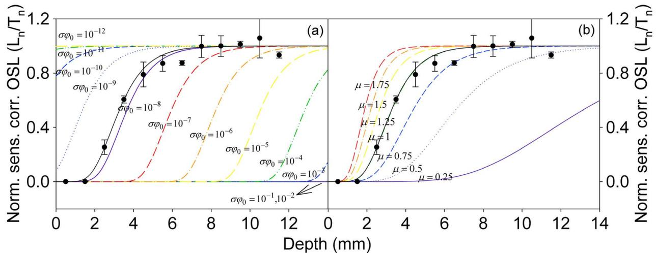
**Figure 4.** Dependence of the model on the involved parameters (a)  $\overline{\sigma\varphi_0}$  and (b)  $\mu$ . The OSL-depth curves vary significantly with the parameter values. The experimental data measured from the known-age road-cut sample are shown as filled circles for comparison.
