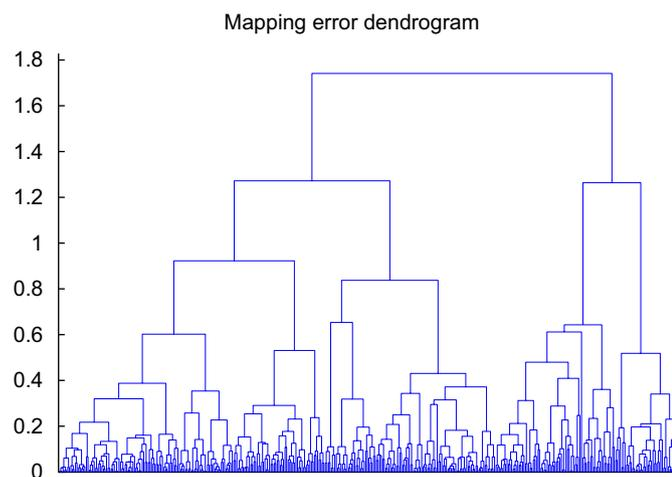
Fig. 4. Mapping error dendrogram. The horizontal axis is the error cluster index, and the vertical axis is the distance between the two error clusters it links. Large values on  $y$  axis indicate that the two linked clusters are quite different; while small values mean that the two linked clusters are similar.
