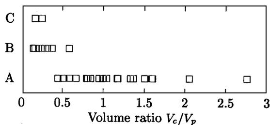
**Fig. 3.** When the instability occurs, one of three possible configurations of the bubbles is found. We plot the occurrence of each of the arrangements A, B and C as a function of the ratio of bubble volumes  $V_c/V_p$ . They are illustrated in Figure 4. For  $V_c > V_p$  configuration A is always obtained, whereas for small  $V_c/V_p$  we see either B or C.
