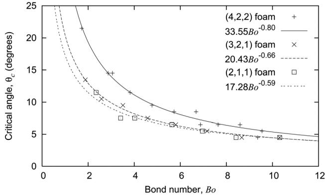
**FIG. 6.** We find the critical angle  $\theta_c$  which is the maximum value for  $\theta$  [see Fig. 1(d)] before the sphere falls out of the foam to touch the cylinder wall. The critical tilt angle for the staircase, chiral and double staircase foams decreases with increasing Bond number. The given fits to a power-law have an exponent that increases with  $\lambda$ .
