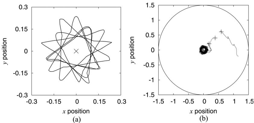
**FIG. 5.** Sphere motion in a chiral foam, with  $Bo = 2.58$ . (a) The path of a sphere which is initially positioned at the center of the top of the cylinder, viewed from above. (b) Tracking the path of the same sphere from three different, noncentral, initial positions. Each initial position is labeled with a cross. If the sphere starts too far away from the center then it moves towards the wall; otherwise it is brought back to the central region of the foam.
