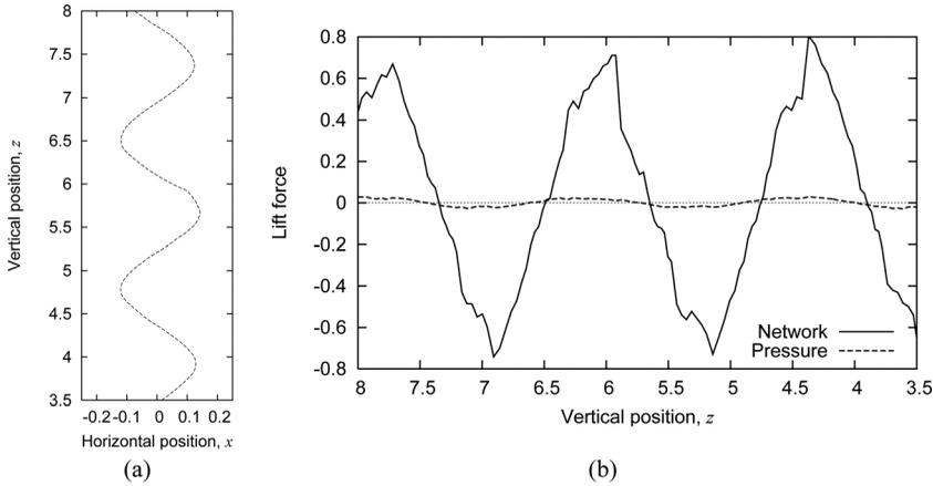
**FIG. 3.** Motion of a sphere in a staircase foam, in the case  $Bo = 2.34$ . (a) The position of the sphere oscillates in the  $(x, z)$  plane, here with amplitude  $a = 0.14$ . (b) The network and pressure components of the (horizontal) lift force exerted on the sphere *versus* its vertical position.
