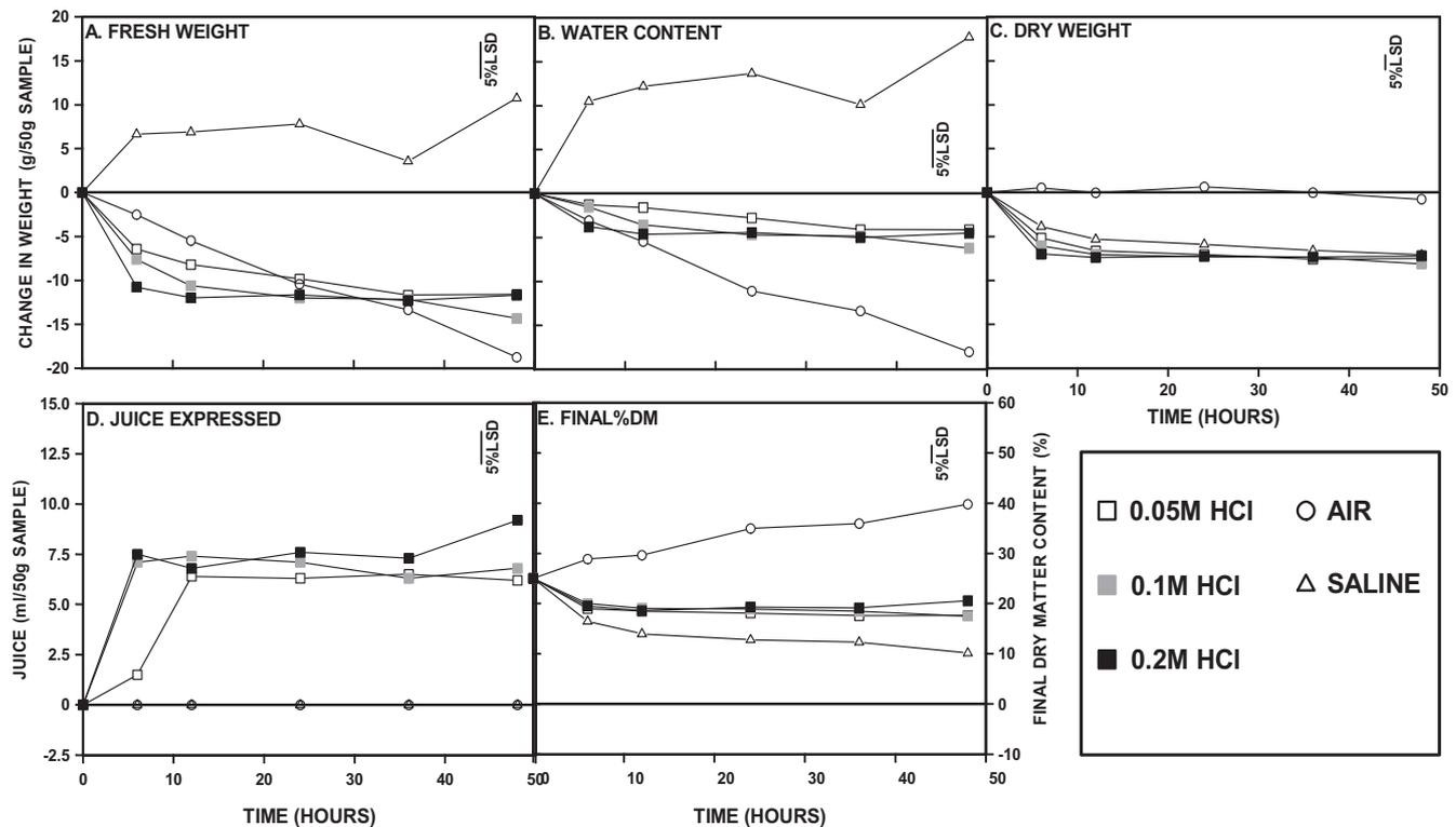
**Fig. 4.** Time-scale of treatment effects on kelp over a 48 h period. A. Fresh weight (g/50 g sample), B. Water content (ml/50 g sample), C. Dry weight (g/50 g sample), D. Juice production in a screw-press (ml/50 g sample) and E. Final DM content (%). 0.05 M hydrochloric acid, open squares; 0.1 M hydrochloric acid, grey squares; 0.2 M hydrochloric acid, black squares; air drying, open circles; saline, open triangles. Data are interaction means (n = 3) and the 5%LSD is indicated.
