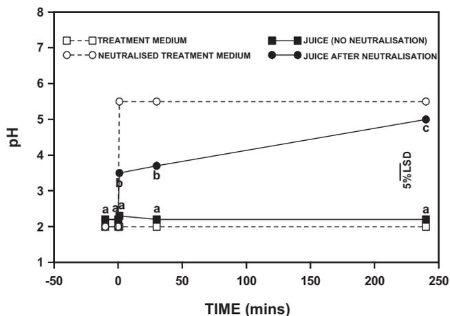
**Fig. 5.** Effect of neutralising the hydrochloric acid treatment medium on the pH of juice produced during screw-pressing. Treatment media, open symbols with dashed lines; juice, closed symbols with continuous lines; squares, acid media; circles, with neutralisation at time zero. Data are interaction means ( $n = 3$ ) and the 5%LSD is indicated. Juice pH data points marked by the same letter are not significantly different at the 5% level as analysed by the Tukey multiple comparison test.
