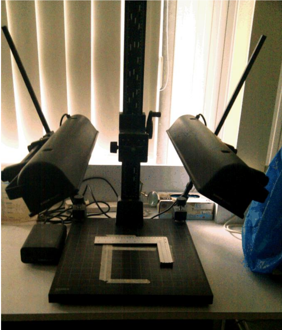
Figure 2: A stable camera setup, with four fluorescent lights, shining onto a copy stand with a setsquare stuck to it to keep square dishes in the same place. A DSLR camera was attached to the screw thread in the centre of the image to photograph the seed.
