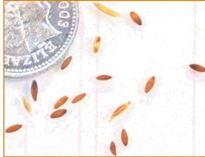
Figure 3-2: Miscanthus seed in a Petri dish (with a 10p coin for scale) to assess FIJI's ability to detect Miscanthus seed, compared to that of a human.
