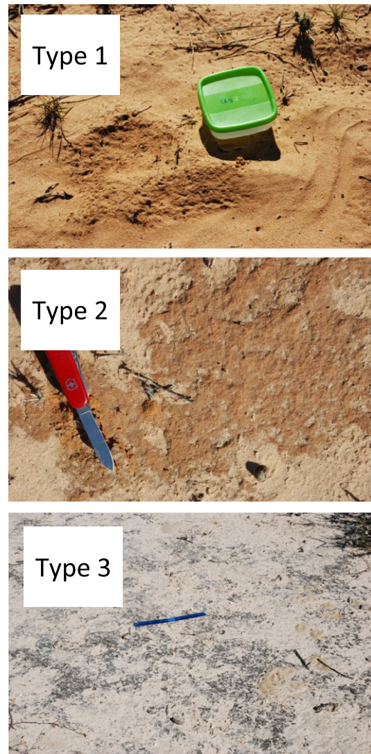
Fig. 1. Photographs showing various crusts Types (1–3) found in Kalahari. The order of their fragility is Type1 > Type2 > Type3. The Types 2 and 3 were used for this study.
